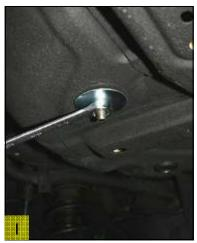
14. Use appropriate caulking, or similar sealant, to seal around the head of the bolt and bracket, as well as around the nut and washer underneath the mounting plate, to prevent exhaust fumes from entering the vehicle.
